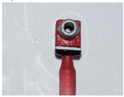
9. Install LEDs inside housing through the bottom with a small amount of clear white glue and test them. Allow to fully cure.
