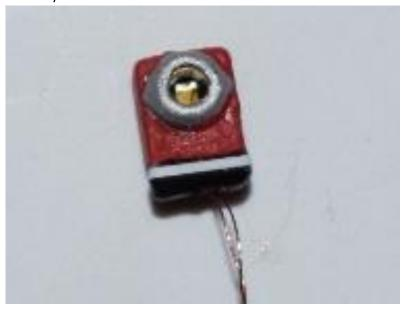
10. Install light lenses with clear white glue. Allow to fully cure.
